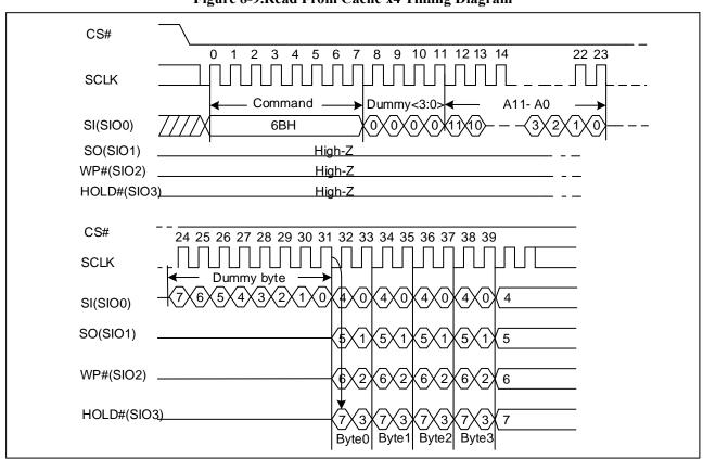
Figure 8-9.Read From Cache x4 Timing Diagram
