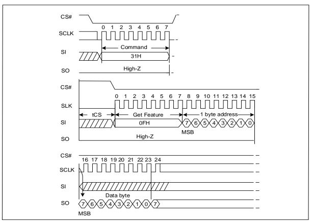
Figure 8-3.Page Read to cache Timing Diagram
