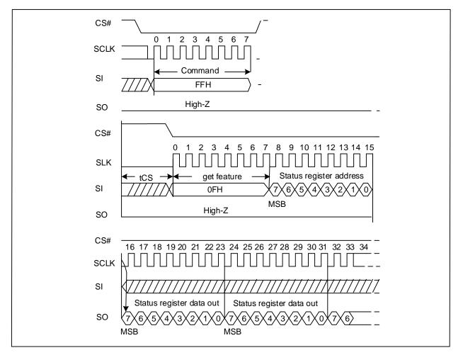
Figure 11-1. Reset Timing Diagram
