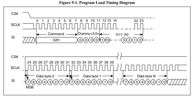
Note: When internal ECC disabled the Data Byte is 2176, when internal ECC enabled the Data Byte is 2112.
