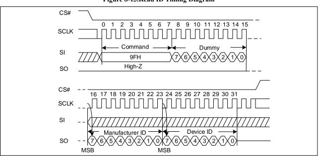
Figure 8-13.Read ID Timing Diagram
