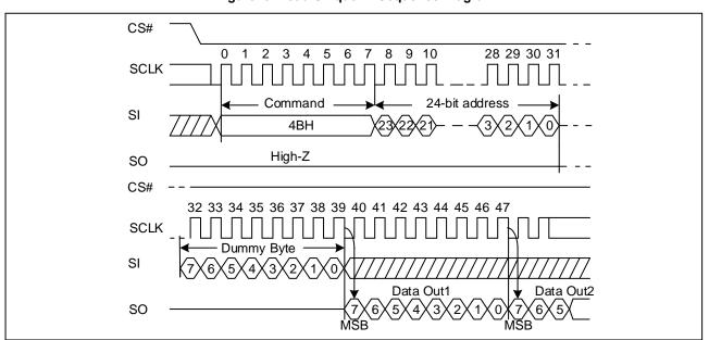
Figure 18. Read Unique ID Sequence Diagram
