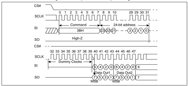
Figure 7. Dual Output Fast Read Sequence Diagram
