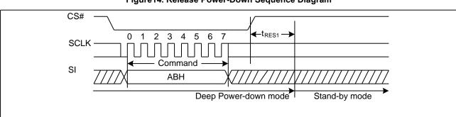
Figure 14. Release Power-Down Sequence Diagram
