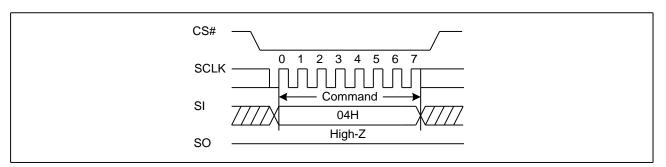
Figure 2. Write Disable Sequence Diagram
