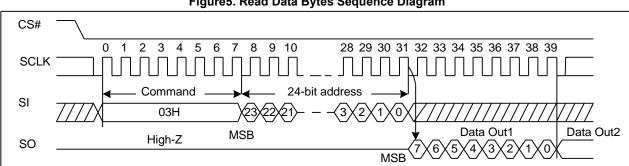
Figure 5. Read Data Bytes Sequence Diagram
