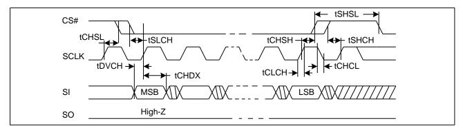
Figure 23. Output Timing
