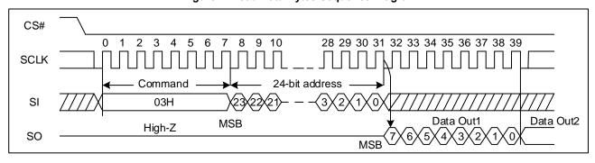
Figure 7. Read Data Bytes Sequence Diagram
