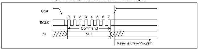
Figure 30. Program/Erase Resume Sequence Diagram
