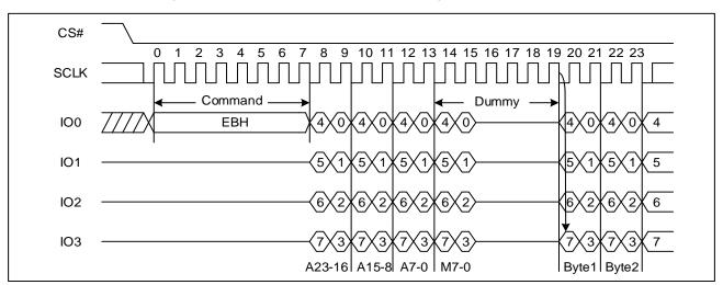
Figure 13. Quad I/O Fast Read Sequence Diagram ((M5-4) ≠ (1, 0))
