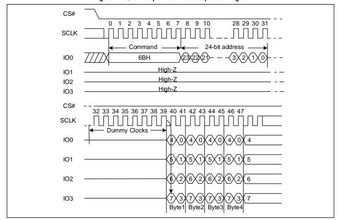
Figure 10. Quad Output Fast Read Sequence Diagram
