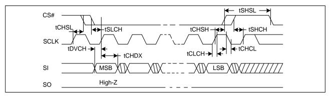
Figure 39. Output Timing
