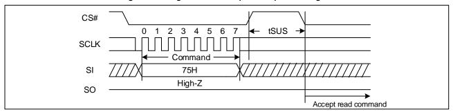
Figure 29. Program/Erase Suspend Sequence Diagram
