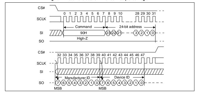
Figure 22. Read Manufacture ID/ Device ID Sequence Diagram
