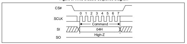
Figure 3. Write Disable Sequence Diagram
