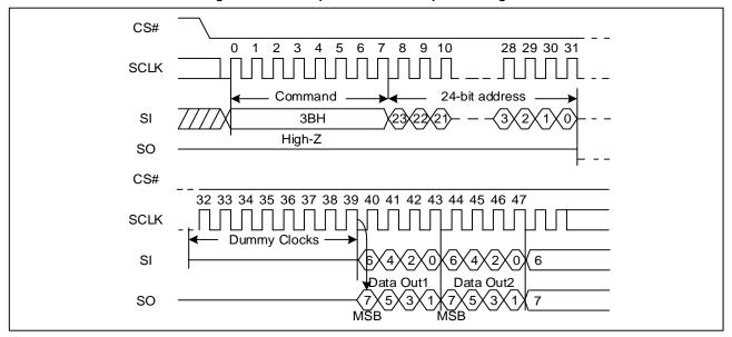
Figure 9. Dual Output Fast Read Sequence Diagram
