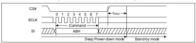
Figure 32. Release Power-Down Sequence Diagram
