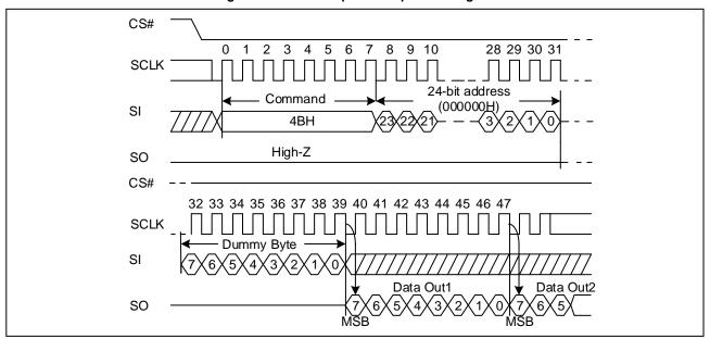
Figure 24. Read Unique ID Sequence Diagram
