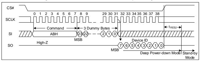
Figure 33. Release Power-Down/Read Device ID Sequence Diagram
