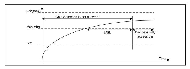
Table 10. Power-Up Timing and Write Inhibit Threshold
