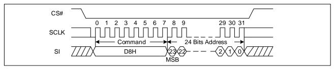
Figure 20. 64KB Block Erase Sequence Diagram
