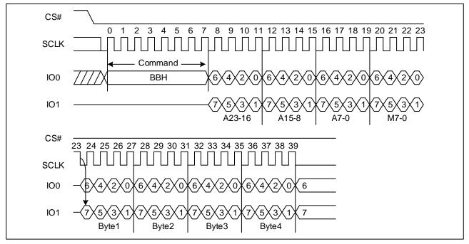
Figure 11. Dual I/O Fast Read Sequence Diagram ((M5-4) ≠ (1, 0))
