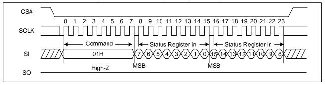
Figure 5. Write Status Register Sequence Diagram
