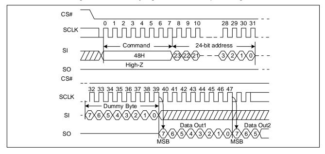
Figure 27. Read Security Registers command Sequence Diagram
