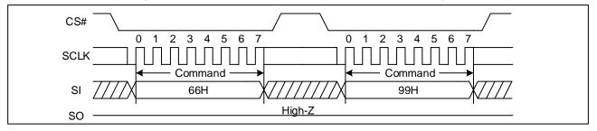
Figure 28. Enable Reset and Reset command Sequence Diagram
