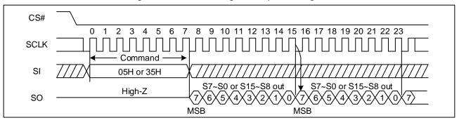
Figure 4. Read Status Register Sequence Diagram
