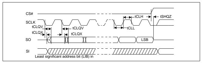
Figure 40. Resume to Suspend Timing Diagram
