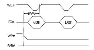
Figure 7-5\_d: Write Protect Enable with erase figures
