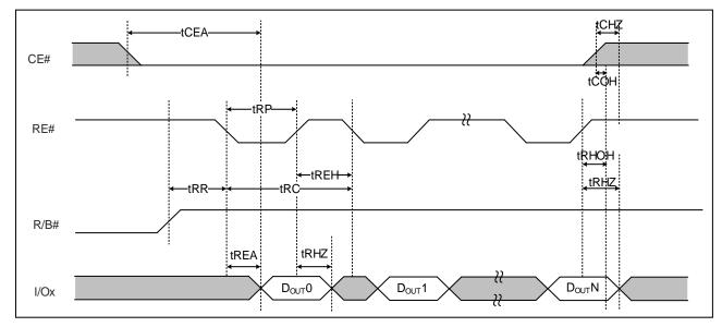
Figure 7-4\_a: Data Output Cycle figures
