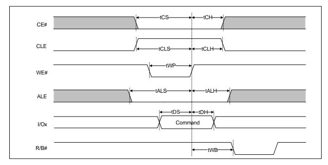
Figure 7-1: Command Input Cycle figures
