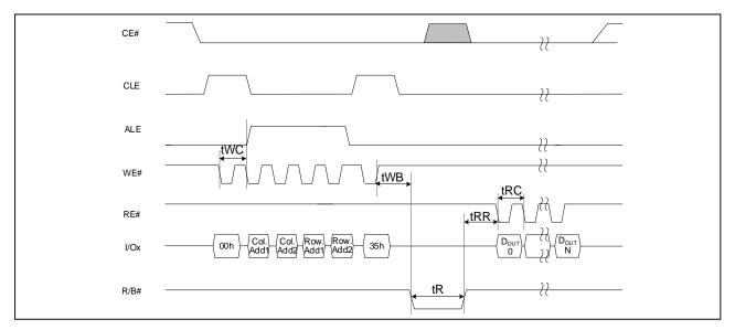
Figure 8-5: Copy-Back read sequential figures
