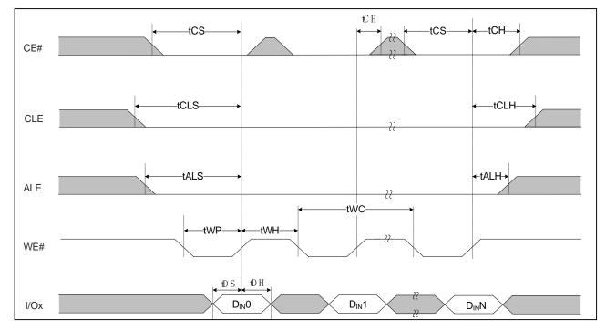
Figure 7-3: Data Input Cycle figures
