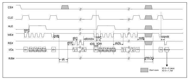
Figure 8-9: Copy-Back Program with Random Data Input figures
