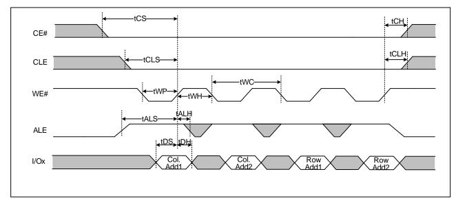
Figure 7-2: Address Input Cycle figures
