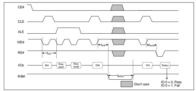
Figure 8-10: Common Block Erase Operation figures
