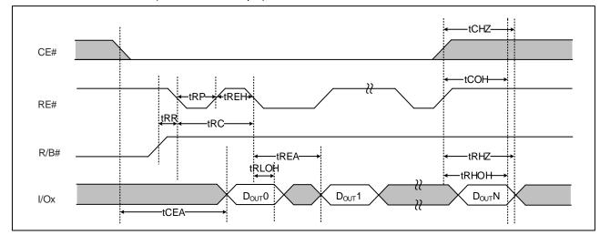
Figure 7-4\_b: Data Output Cycle figures
