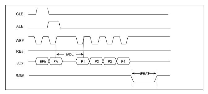
Figure 8-17: Set Feature (EFH) sequential figures
