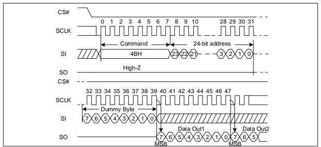
Figure 68 Read Unique ID Sequence Diagram (SPI)
