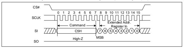
Figure 22 Write Extended Address Register Sequence Diagram (SPI)
