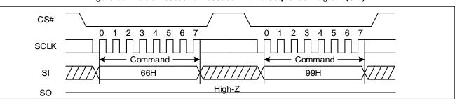
Figure 93 Enable Reset and Reset command Sequence Diagram (SPI)
