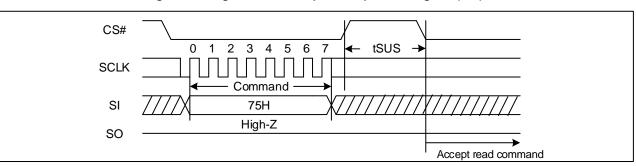
Figure 73 Program/Erase Suspend Sequence Diagram (SPI)
