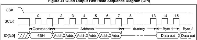
Figure 41 Quad Output Fast Read Sequence Diagram (QPI)
