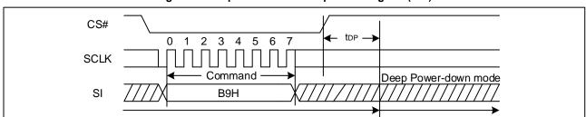
Figure 64 Deep Power-Down Sequence Diagram (SPI)
