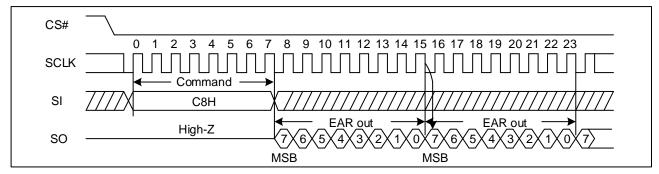
Figure 35 Read Extended Address Register Sequence Diagram (QPI, fsclk <104MHz)
