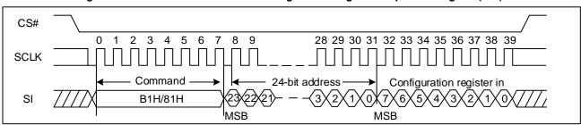
Figure 24 Write Nonvolatile/Volatile Configuration Register Sequence Diagram (SPI)
