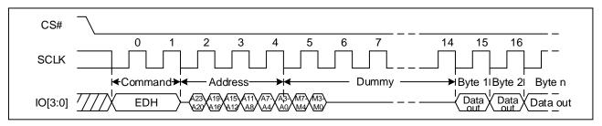
Figure 26. DTR Quad I/O Fast Read Sequence Diagram ((M5-4) = (1, 0))
