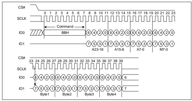
Figure 18. Dual I/O Fast Read Sequence Diagram ((M5-4) ≠ (1, 0))
