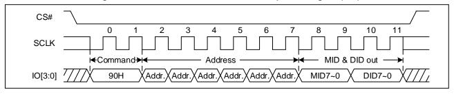
Figure 41. Read Manufacture ID/ Device ID Sequence Diagram (QPI)
