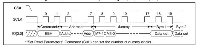
Figure 22 Quad I/O Fast Read Sequence Diagram (M5-4 = (1, 0))
