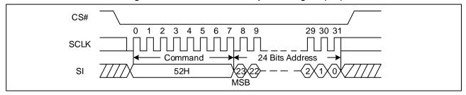
Figure 35. 32KB Block Erase Sequence Diagram (QPI)
