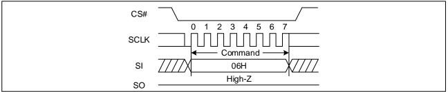
Figure 4. Write Enable Sequence Diagram (QPI)
