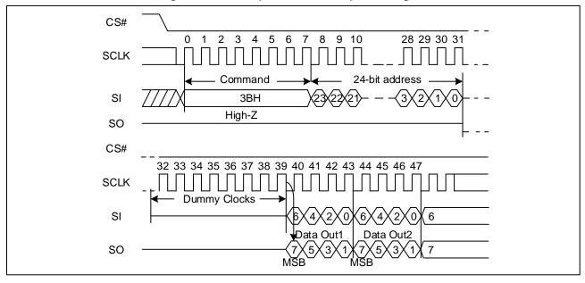
Figure 16. Dual Output Fast Read Sequence Diagram
