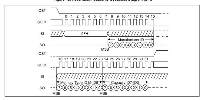
Figure 42. Read Identification ID Sequence Diagram (SPI)
