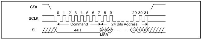
Figure 45. Erase Security Registers command Sequence Diagram
