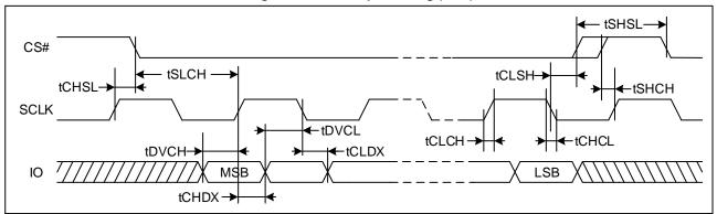
Figure 70. Serial Output Timing (DTR)
