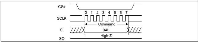
Figure 6. Write Disable Sequence Diagram (QPI)
