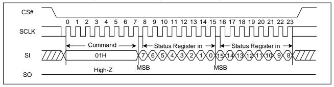
Figure 10. Write Status Register Sequence Diagram (QPI)
