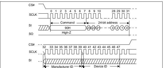
Figure 40. Read Manufacture ID/ Device ID Sequence Diagram (SPI)
