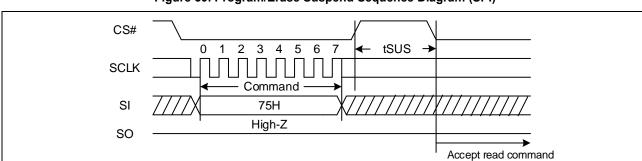
Figure 50. Program/Erase Suspend Sequence Diagram (SPI)
