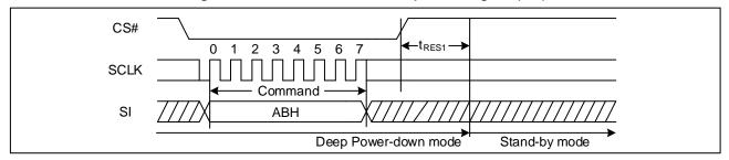
Figure 57. Release Power-Down Sequence Diagram (QPI)
