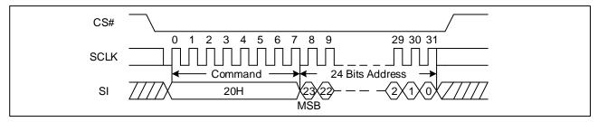
Figure 33. Sector Erase Sequence Diagram (QPI)
