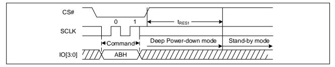
Figure 58. Release Power-Down/Read Device ID Sequence Diagram (SPI)
