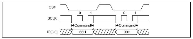
Note: Enable Reset (66H) and Reset (99H) commands cannot reset the device when the device is in Quad I/O DTR Continuous Read Mode. The only way to quit the Quad I/O DTR Continuous Read Mode is to set the "Continuous Read Mode" bits (M5-4) not equal to (1,0).
