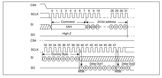
Figure 63. Read Serial Flash Discoverable Parameter command Sequence Diagram (QPI)
