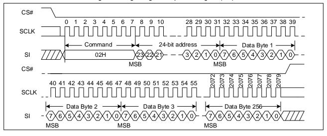
Figure 29. Page Program Sequence Diagram (SPI)
