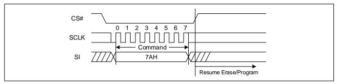
Figure 53. Program/Erase Resume Sequence Diagram (QPI)
