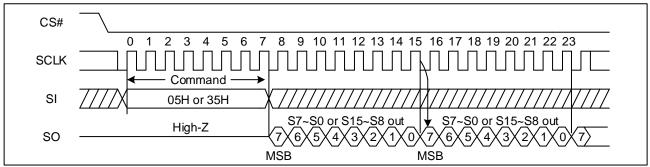
Figure 8. Read Status Register Sequence Diagram (QPI)
