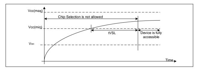
Table 10. Power-Up Timing and Write Inhibit Threshold
