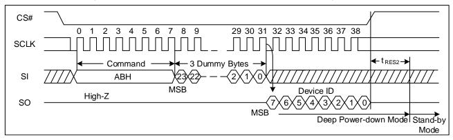
Figure 59. Release Power-Down/Read Device ID Sequence Diagram (QPI)
