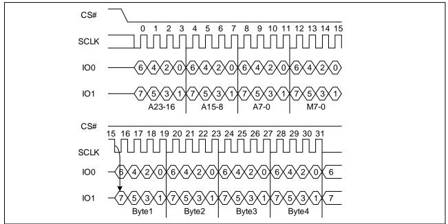
Figure 19. Dual I/O Fast Read Sequence Diagram ((M5-4) = (1, 0))
