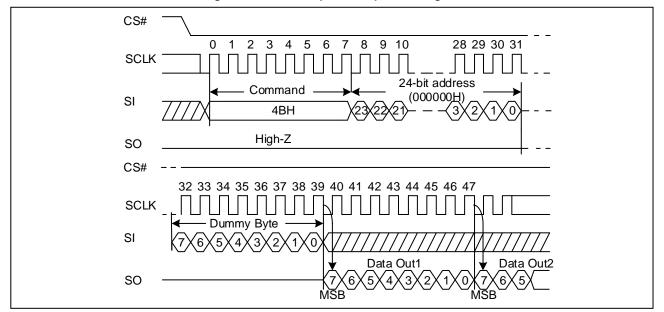
Figure 44. Read Unique ID Sequence Diagram
