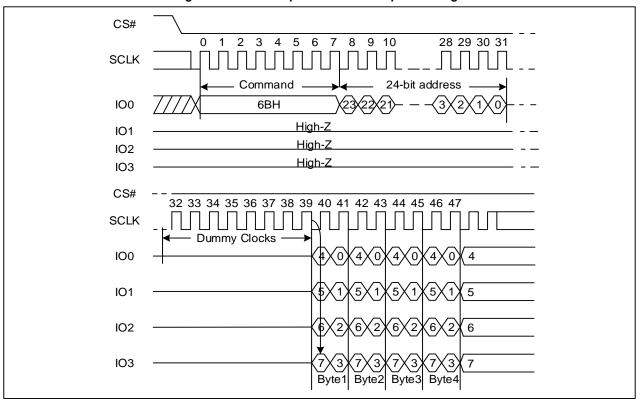
Figure 17. Quad Output Fast Read Sequence Diagram
