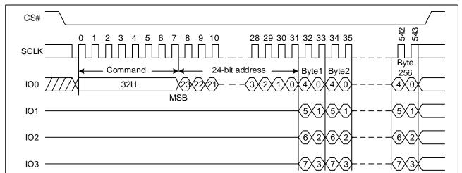
Figure 31. Quad Page Program Sequence Diagram
