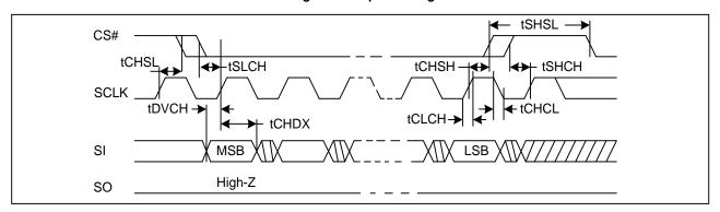
Figure 68. Output Timing
