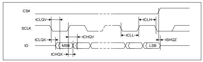
Figure 71. Resume to Suspend Timing Diagram
