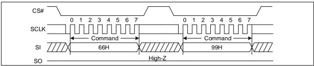
Figure 30. Enable Reset and Reset command Sequence Diagram
