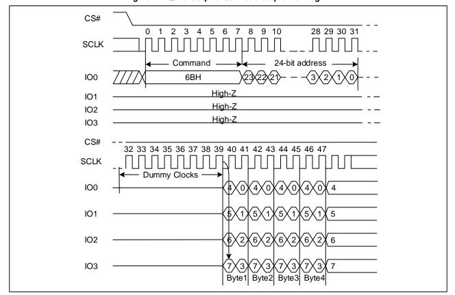
Figure 12. Quad Output Fast Read Sequence Diagram
