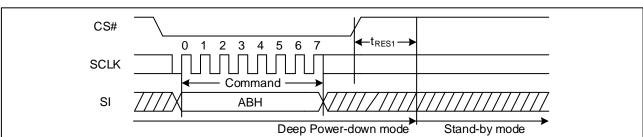
Figure 34. Release Power-Down Sequence Diagram
