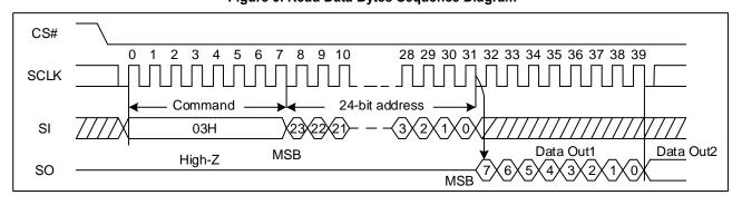
Figure 9. Read Data Bytes Sequence Diagram
