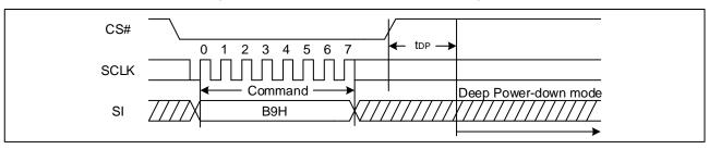
Figure 33. Deep Power-Down Sequence Diagram
