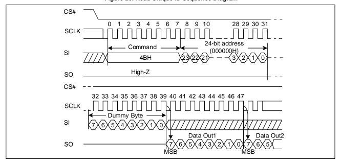
Figure 26. Read Unique ID Sequence Diagram
