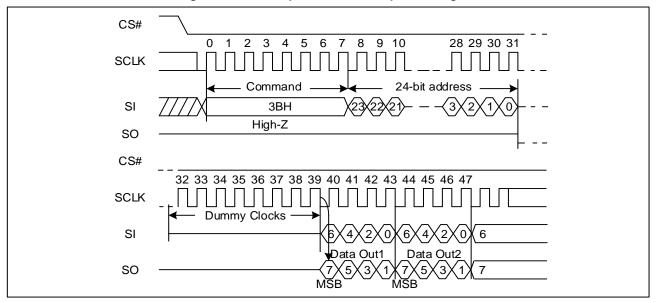
Figure 11. Dual Output Fast Read Sequence Diagram
