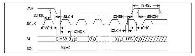
Figure 41. Output Timing
