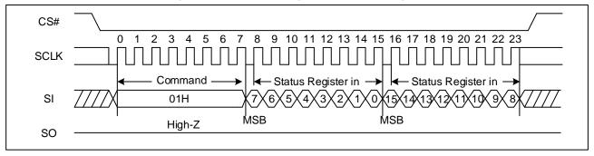
Figure 7. Write Status Register Sequence Diagram
