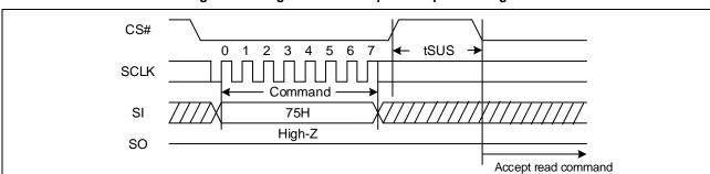
Figure 31. Program/Erase Suspend Sequence Diagram
