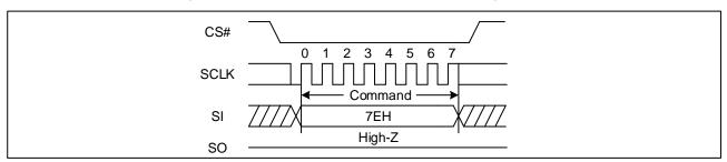
Figure 89 Global Block/Sector Lock Sequence Diagram (QPI)
