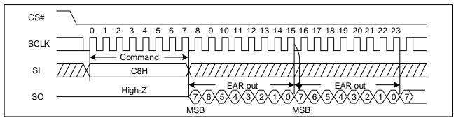
Figure 34 Read Extended Address Register Sequence Diagram (QPI, fsclk≤104MHz)
