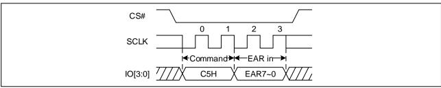
Figure 22 Write Extended Address Register Sequence Diagram (QPI)
