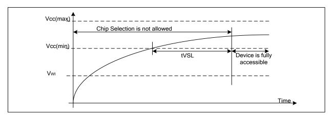
**Table 16 Power-Up Timing and Write Inhibit Threshold**
