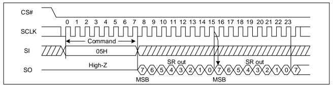
Figure 26 Read Status Register Sequence Diagram (QPI, fsclk≤104MHz)
