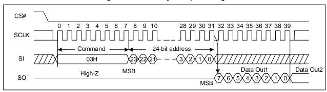
Figure 36 Read Data Bytes Sequence Diagram
