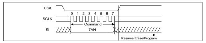
Figure 75 Program/Erase Resume Sequence Diagram (QPI)
