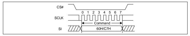
Figure 60 Chip Erase Sequence Diagram (QPI)
