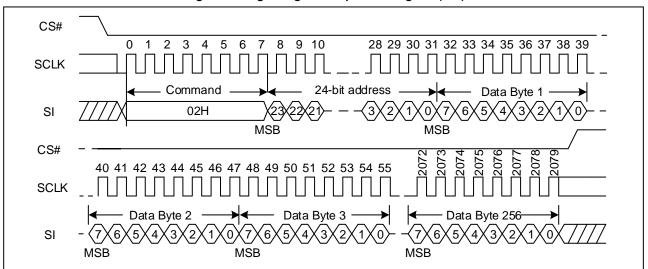
Figure 47 Page Program Sequence Diagram (SPI)
