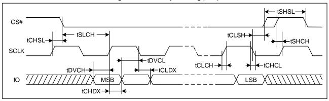
Figure 102. Serial Output Timing (DTR)
