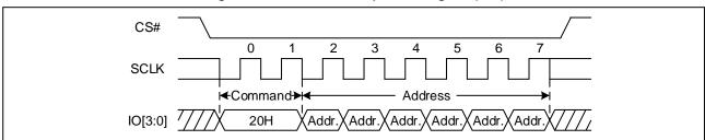
Figure 54 Sector Erase Sequence Diagram (QPI)
