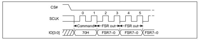
Figure 30 Read Flag Status Register Sequence Diagram (QPI, f<sub>SCLK</sub> > 104MHz)
