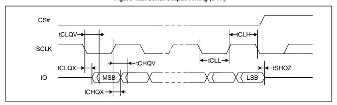
Figure 103. Resume to Suspend Timing Diagram
