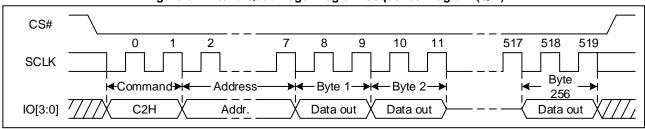
Figure 52 Extend Quad Page Program Sequence Diagram (QPI)
