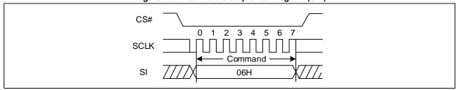
Figure 14 Write Enable Sequence Diagram (QPI)
