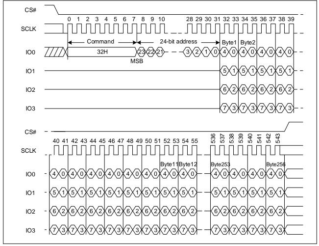
Figure 49 Quad Page Program Sequence Diagram (SPI)
