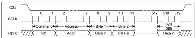
Figure 79 Program Security Registers command Sequence Diagram (QPI)
