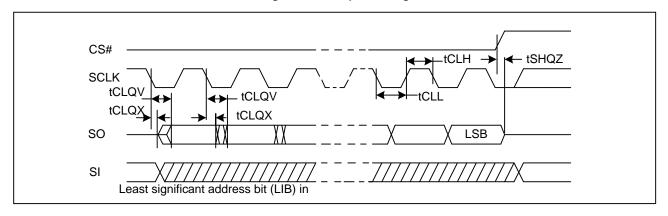
Figure 101. Serial Input Timing (DTR)
