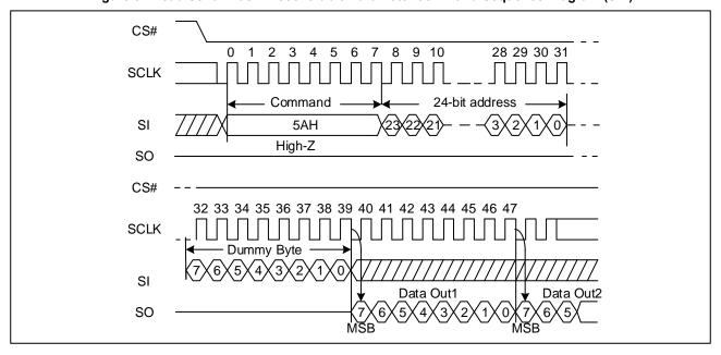
Figure 95 Read Serial Flash Discoverable Parameter command Sequence Diagram (QPI)
