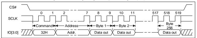
Figure 50 Quad Page Program Sequence Diagram (QPI)
