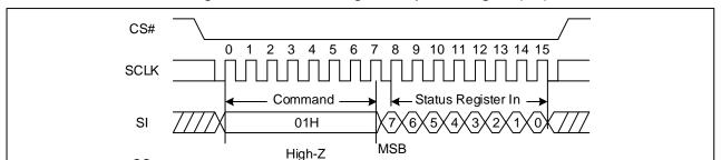
Figure 19 Write Status Register Sequence Diagram (SPI)
