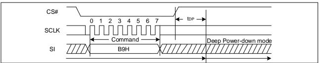
Figure 64 Deep Power-Down Sequence Diagram (QPI)
