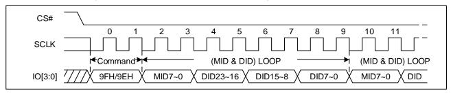
Figure 71 Read Identification ID Sequence Diagram (QPI, fsclk > 104MHz)
