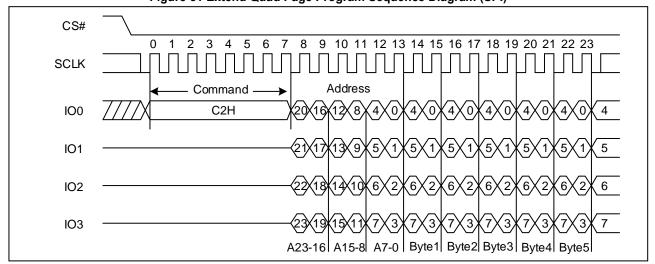
Figure 51 Extend Quad Page Program Sequence Diagram (SPI)
