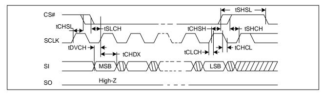
Figure 100. Output Timing
