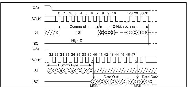
Figure 67 Read Unique ID Sequence Diagram (SPI)
