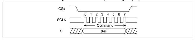
Figure 16 Write Disable Sequence Diagram (QPI)
