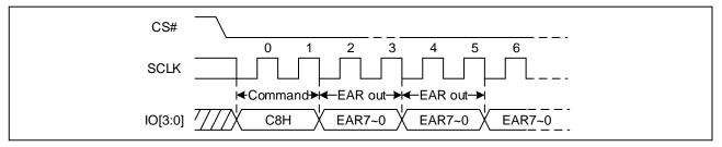
Figure 35 Read Extended Address Register Sequence Diagram (QPI, f<sub>SCLK</sub> > 104MHz)
