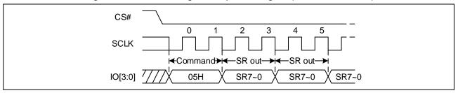
Figure 27 Read Status Register Sequence Diagram (QPI, fsclk > 104MHz)
