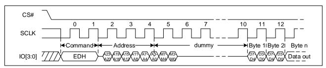
Figure 45. DTR Quad I/O Fast Read Sequence Diagram (QPI, M5-4 ≠ (1, 0))
