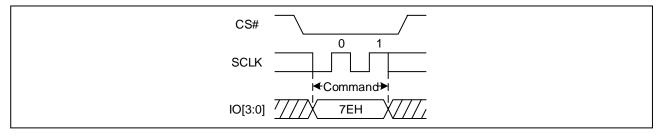
Figure 90 Global Block/Sector Unlock Sequence Diagram (SPI)
