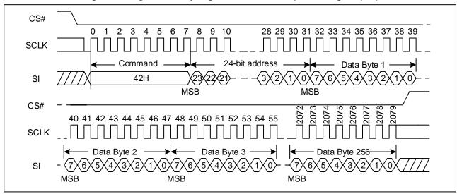
Figure 78 Program Security Registers command Sequence Diagram (SPI)
