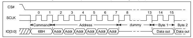
Note: The device default is in 24-bit address mode. For 4-Byte mode, the address length becomes 32-bit.
