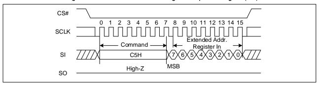
Figure 19 Write Extended Address Register Sequence Diagram (SPI)
