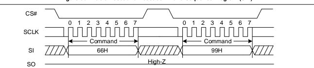
Figure 90 Enable Reset and Reset command Sequence Diagram (SPI)
