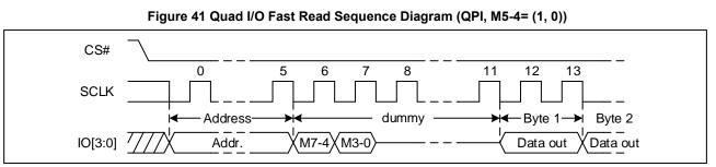
Note: The device default is in 24-bit address mode. For 4-Byte mode, the address length becomes 32-bit.
