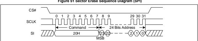
Figure 51 Sector Erase Sequence Diagram (SPI)
