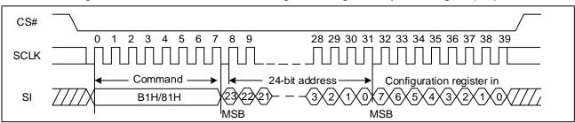
Figure 21 Write Nonvolatile/Volatile Configuration Register Sequence Diagram (SPI)
