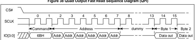
Figure 38 Quad Output Fast Read Sequence Diagram (QPI)
