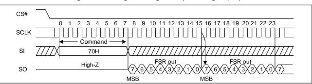
Figure 26 Read Flag Status Register Sequence Diagram (SPI)
