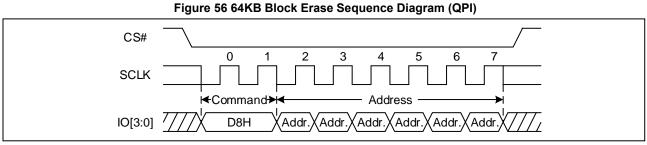
Note: The device default is in 24-bit address mode. For 4-Byte mode, the address length becomes 32-bit.
