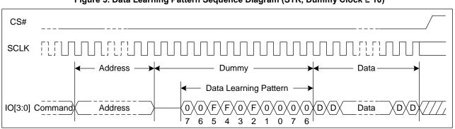
Figure 3. Data Learning Pattern Sequence Diagram (STR, Dummy Clock ≥ 10)
