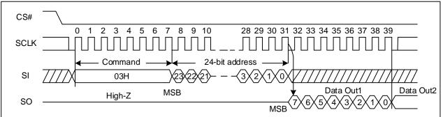
Note: The device default is in 24-bit address mode. For 4-Byte mode, the address length becomes 32-bit.
