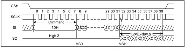
Note: The device default is in 24-bit address mode. For 4-Byte mode, the address length becomes 32-bit. GD55LB02GE-Rev1.4 56
