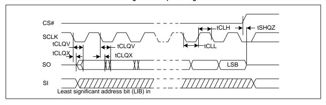
Figure 42. Resume to Suspend Timing Diagram
