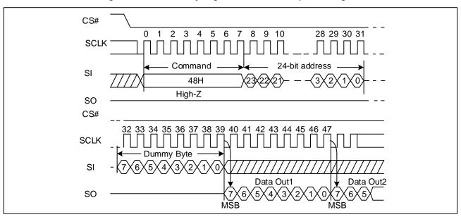
Figure 29. Read Security Registers command Sequence Diagram
