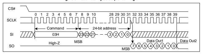
Figure 9. Read Data Bytes Sequence Diagram
