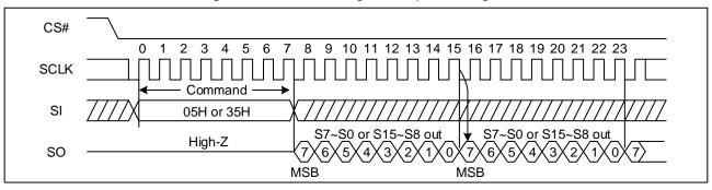
Figure 6. Read Status Register Sequence Diagram
