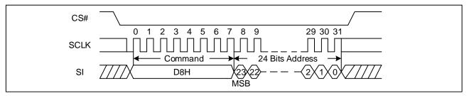
Figure 22. 64KB Block Erase Sequence Diagram
