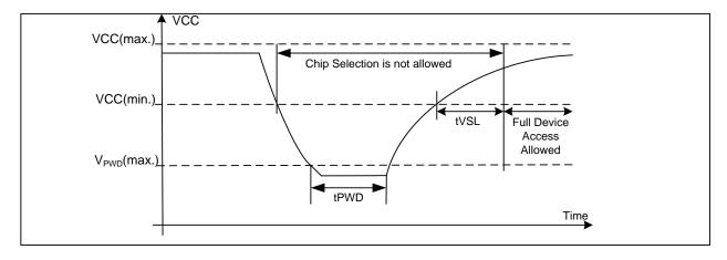
Table 11. Power-Up Timing and Write Inhibit Threshold
