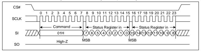
Figure 7. Write Status Register Sequence Diagram
