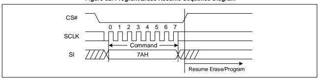
Figure 32. Program/Erase Resume Sequence Diagram
