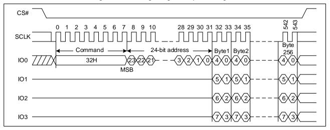
Figure 19. Quad Page Program Sequence Diagram
