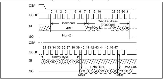
Figure 26. Read Unique ID Sequence Diagram
