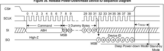
Figure 35. Release Power-Down/Read Device ID Sequence Diagram
