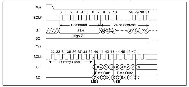
Figure 11. Dual Output Fast Read Sequence Diagram
