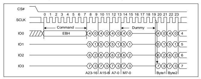
Figure 15. Quad I/O Fast Read Sequence Diagram ((M5-4) ≠ (1, 0))
