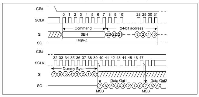
Figure 10. Read Data Bytes at Higher Speed Sequence Diagram
