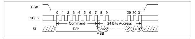
Figure 14. 64KB Block Erase Sequence Diagram
