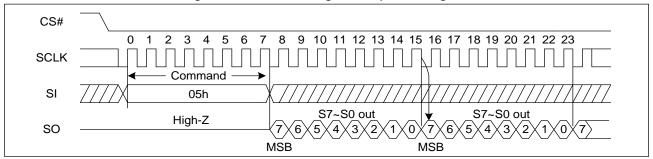
Figure 6. Read Status Register Sequence Diagram
