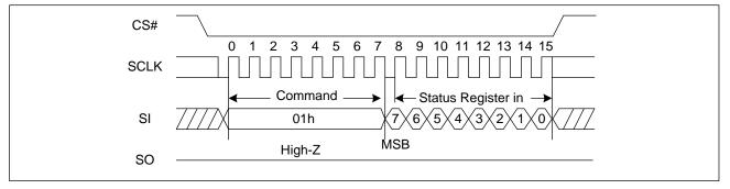
Figure 7. Write Status Register Sequence Diagram
