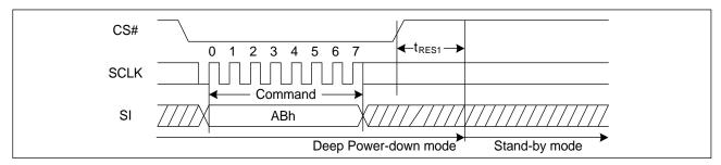
Figure 21. Release Power-Down/Read Device ID Sequence Diagram
