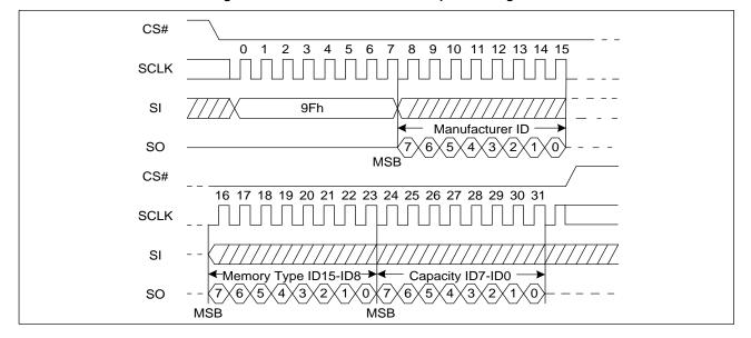
Figure 17. Read Identification ID Sequence Diagram
