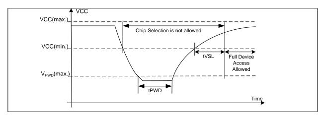
Table 9. Power-Up Timing and Write Inhibit Threshold
