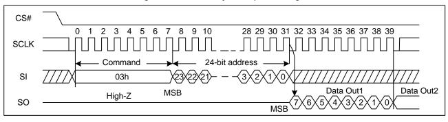
Figure 8. Read Data Bytes Sequence Diagram
