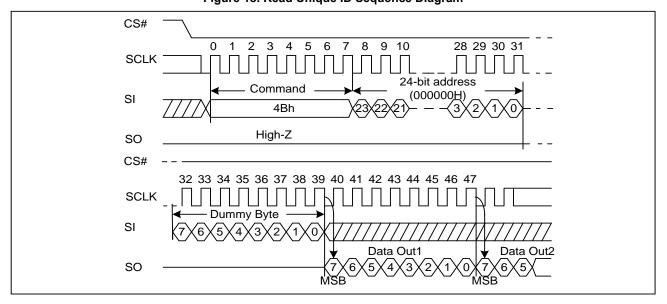
Figure 18. Read Unique ID Sequence Diagram
