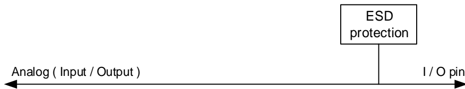
Figure 7-4. Basic structure of Analog configuration
