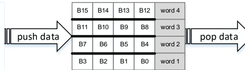
Figure 10-5. Data packing/unpacking when PWIDTH = '01'
