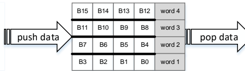
Figure 10-4. Data packing/unpacking when PWIDTH = '00'
