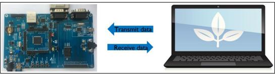
As shown in <u>Figure 3-19. Virtual serial port data interaction</u>, CDC device implemented data callback function. When host sent the data to device, computer software transmit data to OUT endpoint of CDC device through USB bus, OUT endpoint load the received data into application buffer. When device sent the data to host, the data in application buffer is loaded into Tx FIFO, CDC device send the received data to host through IN endpoint, the received data is displayed in HyperTerminal.
