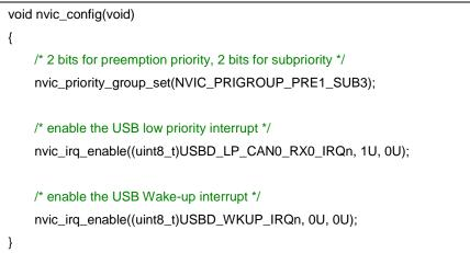
As shown in the <u>Table 2-5. Code table NVIC configuration</u>, considering that USBD interrupt is frequently called, it is necessary to ensure that USBD interrupt are not blocked for a long time in USBD related application. Otherwise, USBD data transmission exceptions possibly occur. Therefore, the interrupt priority of USBD needs to be as high as possible to ensure that the bus is not preempted by other interrupts for a long time.
