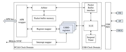
As shown in the *Figure 2-3. USBD RCU domain*, USBD register configuration and other operations are completed under the PCLK clock domain, while data interaction between the USBD device and the host should be completed in the USBD clock domain (48MHz clock).
