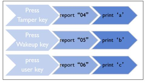
After the enumeration of HID keyboard devices completed, a keyboard device is added to the device manager of the host. As shown in the *Figure 3-6. HID keyboard applicaton* <u>example</u>, Press the Tamper key of the development board, set the value of hid->data [2] to "04", send the message to the host through the device IN endpoint, and the host displays "a"; press the Wakeup key, and the host displays "b"; press the User key, and the host displays "c".
