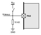
**Note:** In this mode, attention should be paid to the circuit design. If there is a series resistance between the WKUP pin and V<sub>DD</sub>, additional power consumption may be added.
