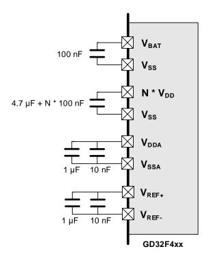
**Note:** All decoupling capacitors must be placed close to the corresponding VDD, VDDA, VREF pins of the chip.
