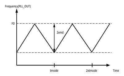
**Note:** If the PLL spread spectrum function is enabled, the system clock frequency will fluctuate, and peripherals that require high clock accuracy may not work properly, such as Ethernet applications that use the MCU IO output clock as the PHY clock and USB related applications.
