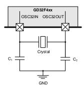
Figure 2-14. LXTAL External Clock Circuit
