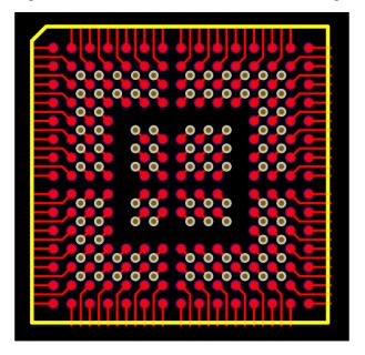
For the BGA package with 0.65 mm pitch, it is recommended to set 4 mil line width and line spacing, and use 8/12 mil (if the overcurrent is large, 8/13 mil can also be used, larger than 8/13 mil size, 4 mil line width line distance from the out-of-line) vias for fan-out, after the fan-out is shown in *Figure 3-7. Fan-Out Method of BGA176 Package*. The via-to-pad distance
