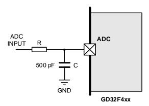
When  $f_{ADC}$  = 40MHz, the relationship between the input impedance and the sampling period is as follows. In order to obtain better conversion results, it is recommended to reduce the frequency of  $f_{ADC}$  as much as possible during use, and select a larger value for the sampling period. When designing external circuits, try to reduce the input Impedance, if necessary, use the op amp to follow to reduce the input impedance.
