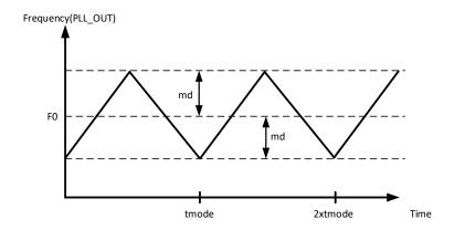
Figure 2-16. Down Spread Spectrum
