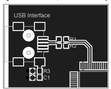
Figure 3-4. Recommend DM, DP Differential Trace Layout Design
