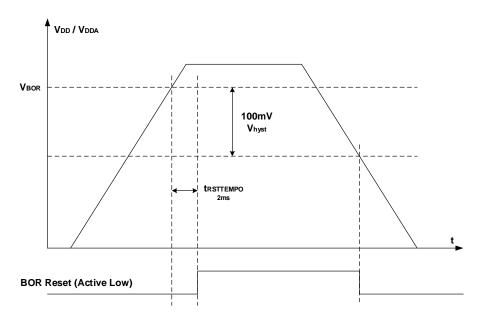
The BOR threshold is set through the option byte BOR\_TH, and can set three different levels.
