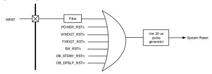
Figure 2-9. Recommend External Reset Circuit
