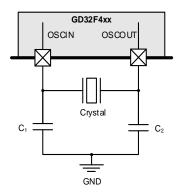
Figure 2-12. HXTAL External Clock Circuit
