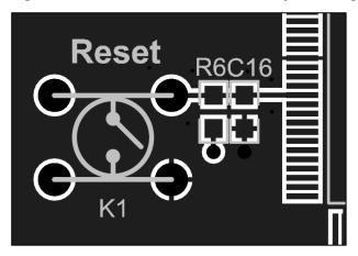
**Note:** The resistance and capacitance of the reset circuit should be as close as possible to the NRST pin of the MCU, and the NRST trace should be kept away from devices with strong
