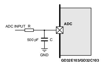
When fADC = 42MHz, the relationship between input impedance and sampling period is as follows. In order to obtain better conversion results, it is recommended to reduce the frequency of fADC as much as possible, and select a larger sampling period as much as possible. In the design of external circuit, input impedance should also be reduced as much as possible.
