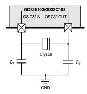
Figure 2-12. LXTAL External Clock Circuit
