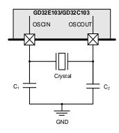
Figure 2-10. HXTAL External Clock Circuit
