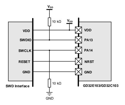
There are several ways to improve the reliability of SWD download and debugging communication and enhance the anti-interference ability of download and debugging.
