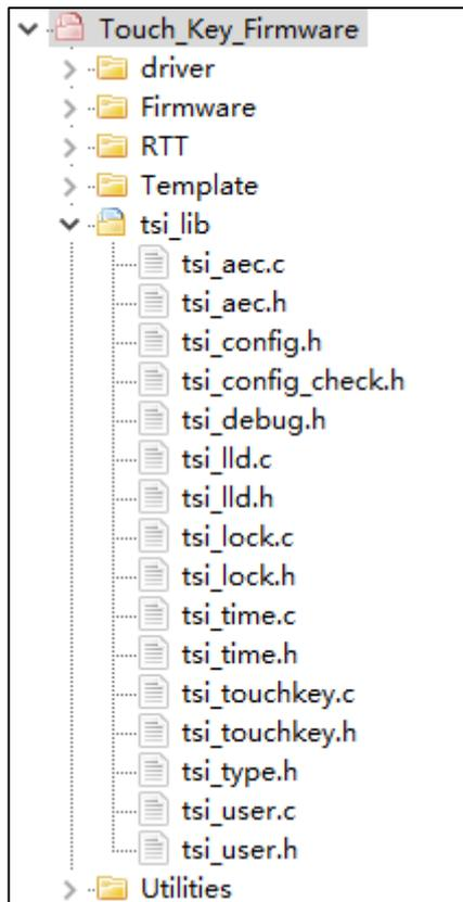
tsi\_aec.c / tsi\_aec.h contains adaptive environment change detection code, which mainly modifies the channel reference value periodically.
