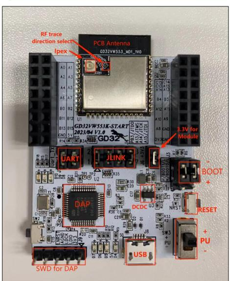
Figure 2-1. Reference connection of GD development board
