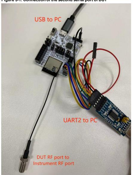
Figure 5-1. Connection of the second serial port of DUT
