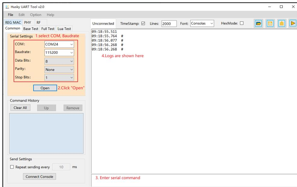
2. Click the button to connect the serial port. Press "Reset" at the side of the development board, and the serial port output box displays the log information, as shown in [Figure 4-2. Serial port boot information](#). At this time, left-click in the serial port input box and press "Enter" on the keyboard, and the log displays "#":
