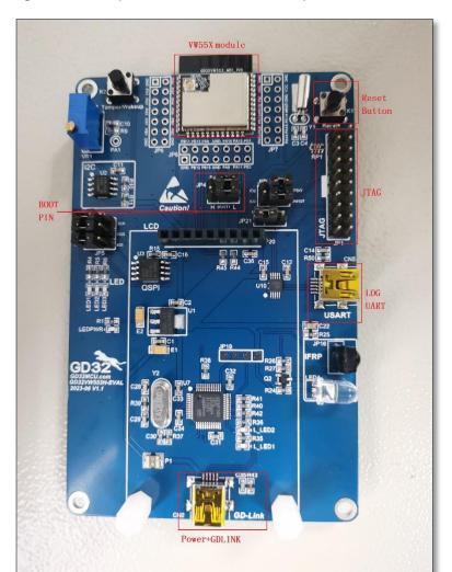
Figure 1-2. The picture of the EVAL development board
