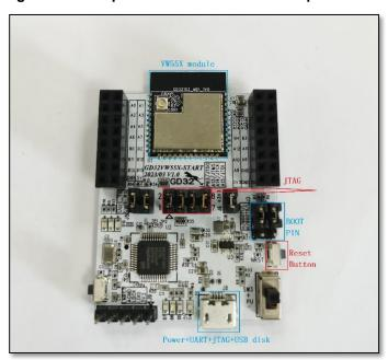
Developers mainly focus on the following parts of the development board, which have been marked in the figure.
